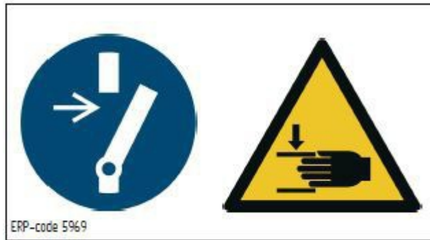
5969 - Warning on inspection door and hinged fan plate
