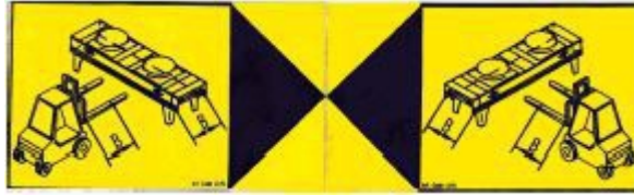
4494 - Range for forklift with positioning marks; for units with up to 2 fans
