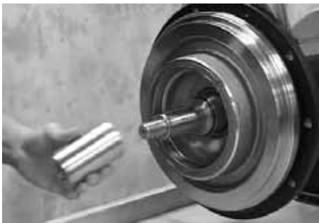
Fig. 13 Removing positioning tool
