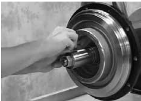
Fig. 12 Tightening shaft seal
