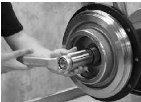
Fig. 11 Positioning tool for primary shaft seal
