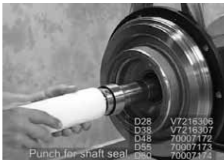
Fig. 7 Punching for shaft seal
