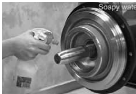
Fig. 4 Lubricating shaft with soapy water
