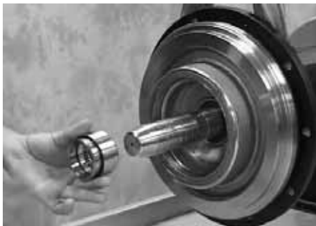
Fig. 6 Fitting shaft seal on shaft
