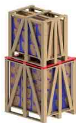
Figure 5.5 - Use of additional battens for stacking
