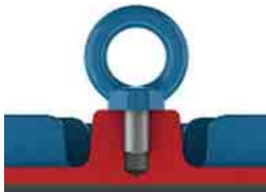
Figure 4.1 - Correct tightening of the eyebolt
