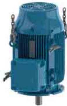
Figure 4.17 - Install the second pair of eyebolts
