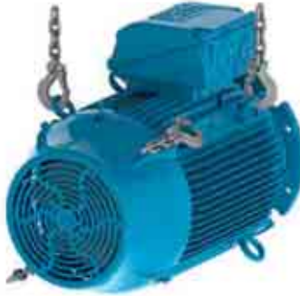
Figure 4.10 - Installation of the second pair of eyebolts
