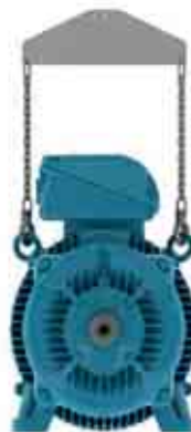
Figure 4.6 - Use of a spreader beam for lifting
