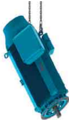
Figure 4.14 - Lifting HGF and W50 motors by the eyebolts at the non-drive end
