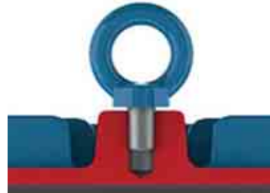
Figure 4.2 - Incorrect tightening of the eyebolt
