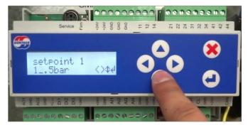
6th STEP: after setpoint value adjustment, press the enter key again. next, press the x key to return to the status menu.
