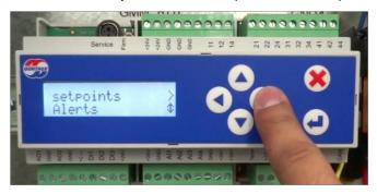
4th STEP: to change the setpoint, press the enter key. therefore, the adjustment of the desired value is enabled.
