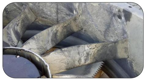
Fan condition before performing the cleaning procedure:
