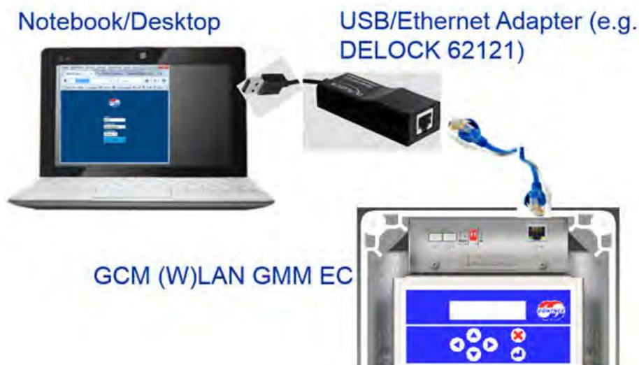
Alternatively, however, you can also use the existing network interfaces on your computer. Establish a direct connection between the computer and GCM (W)LAN for this purpose.
