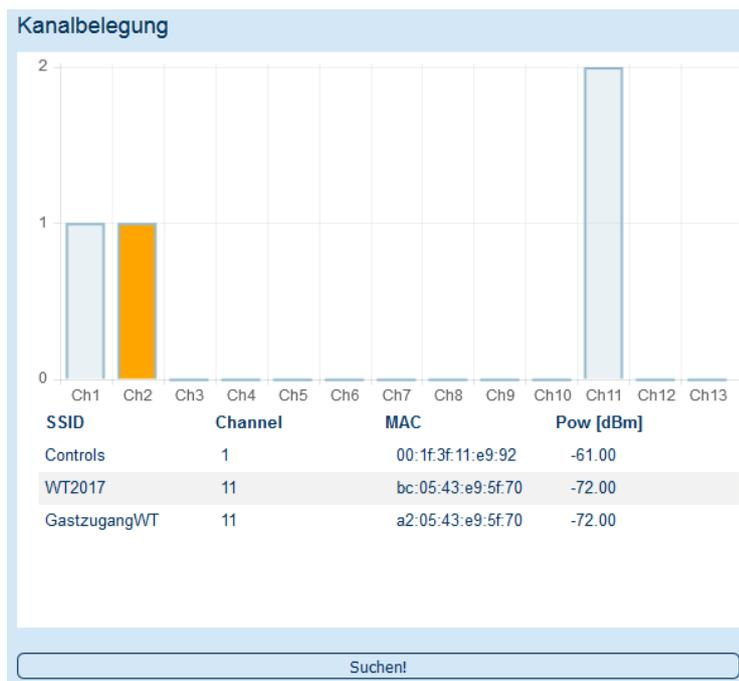
In this specific case, therefore, the GCM-WLAN should be configured to operate in Channel 6 instead of Channel 2.
