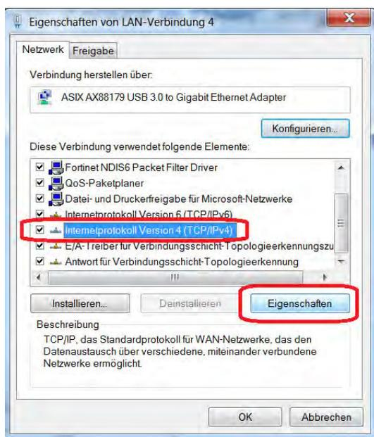
The GCM (W)LAN uses the default IP address 192.168.1.1 in the LAN. In other words, you have to assign your computer an IP address from the same segment.
