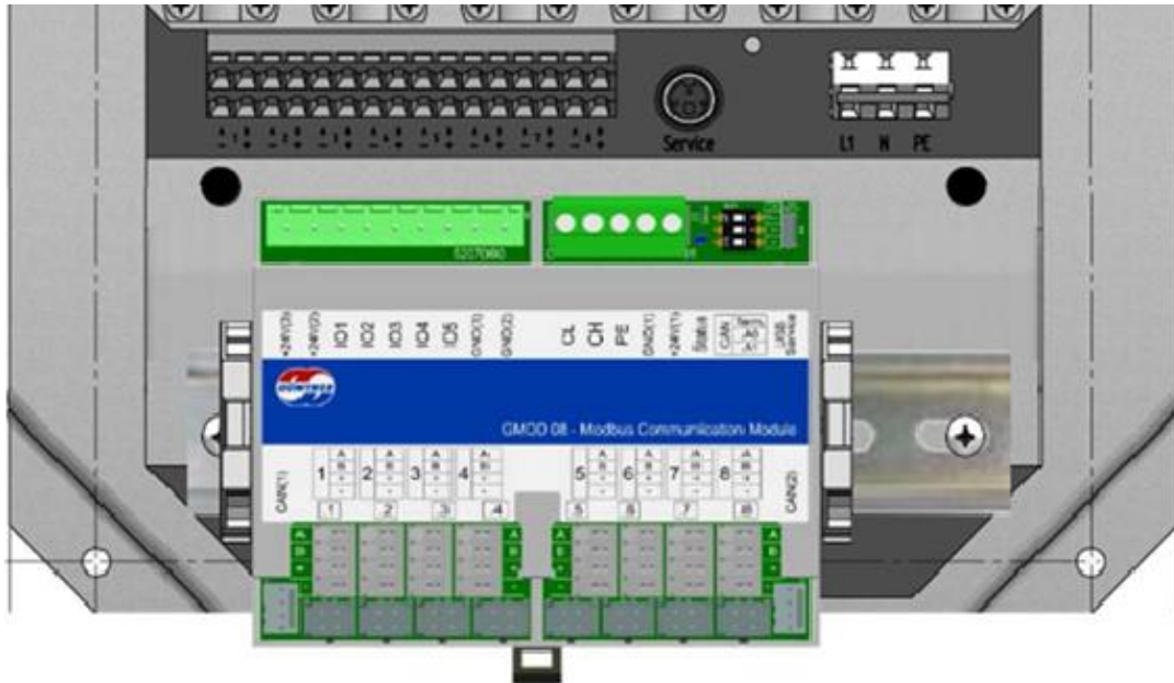
Figure 11: Attaching the GMOD 08 Rail module.
