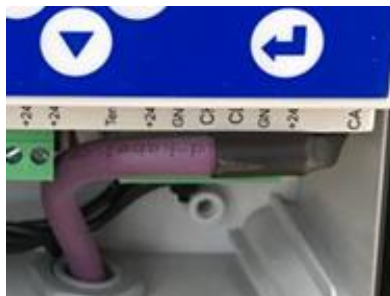
Figure 19: CAN communication cable.
